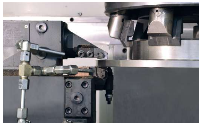
Lift-off slide in turret
