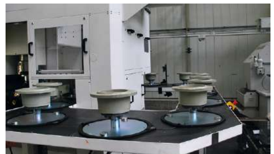
Chain driven conveyor with pallets
