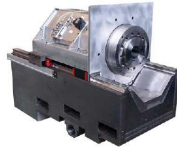
Thermo-symmetrical spindle construction employed consistently in all machines for maximum precision
