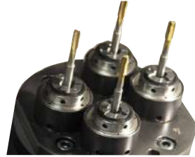
Multiple drill head
