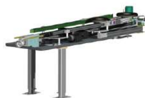
Inverted-tooth chain driven conveyor
