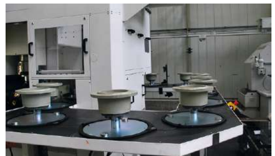
Chain driven conveyor with pallets
