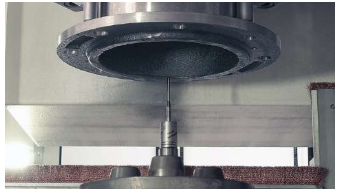
Workpiece gauging can be done in a clean environment outside the work area
