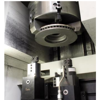
Step 2: Machine 1st side
