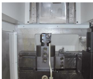
Multifunction plate as a low-cost alternative to the turret (DVT 300)
