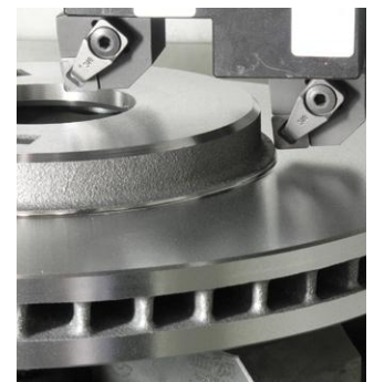
Step 4: Machine 2nd side
