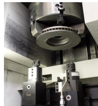
Step 2: Machine 1st side
