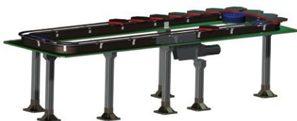
Oval conveyor belt drag conveyor
