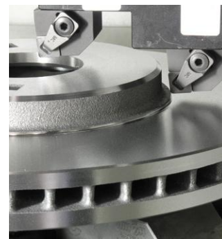
Step 4: Machine 2nd side
