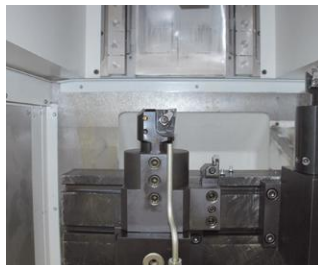
Multifunction plate as a low-cost alternative to the turret (DVT 300)
