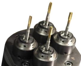
Multiple drill head
