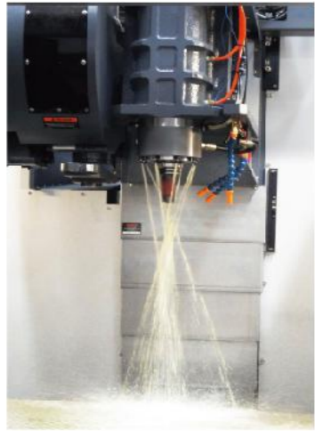
Spindle Annular Coolant Jet with 8 Nozzles
