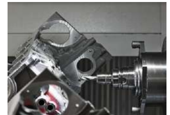
HSK-A63 motor spindle with holder for angular milling head
