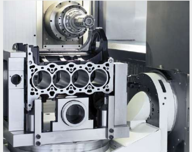
Honing a 4-cylinder crankcase
