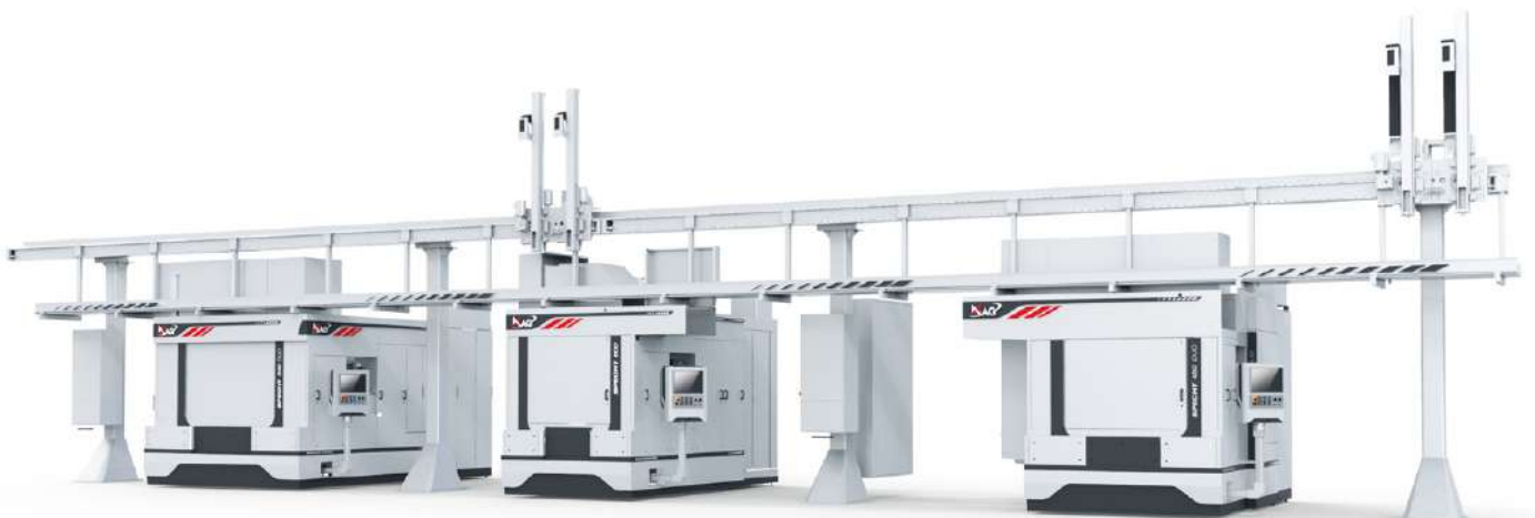
Linked SPECHT® high performance machines with MAG gantry (overhead loading)
