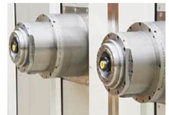
HSK-A100 motor spindles on the SPECHT® DUO
