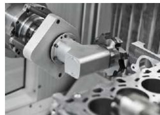
Automatically interchangeable angular milling head
