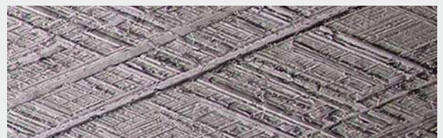
Magnification of a diamond-honed bore surface
