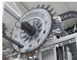
HSK-A100 disc magazin with 26 places
