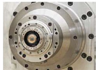
HSK-A63 motor spindle of a SPECHT® single-spindle machine
