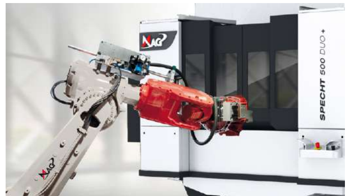
Robot loading on a SPECHT® 500 DUO+
