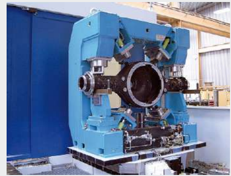
Jig with axle housing
