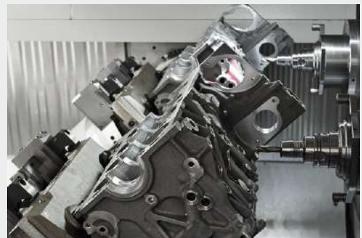
Drilling operations on a cylinder block
