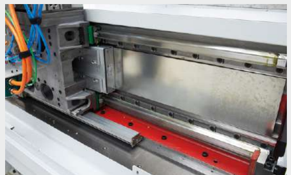
Z axis with linear drive
