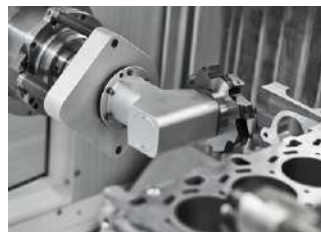
Automatically interchangeable angular milling head
