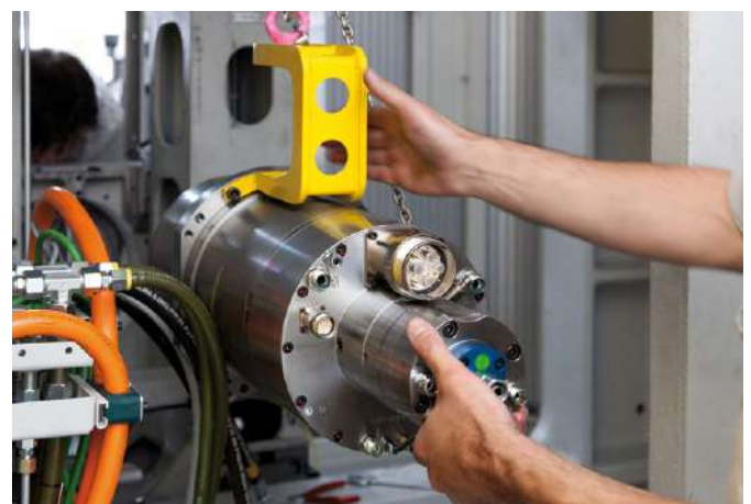
Universal spindle lifting device for single and dual spindle machines
