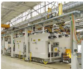
Parallel system that can be loaded by overhead gantries with linear lifting axes or robot arms
