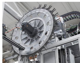
HSK-A100 disc magazin with 26 places
