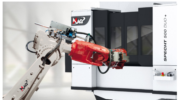
Robot loading on a SPECHT® 500 DUO+
