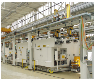
Parallel system that can be loaded by overhead gantries with linear lifting axes or robot arms
