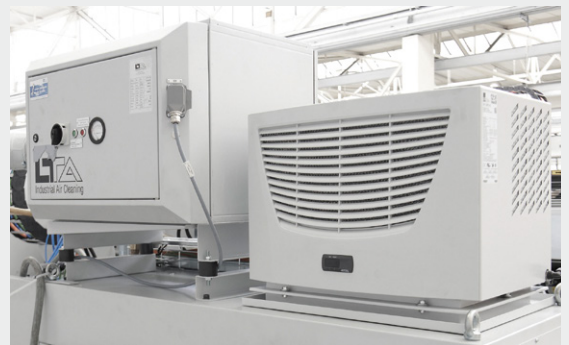
Oil and emulsion mist separators with cabinet cooling
