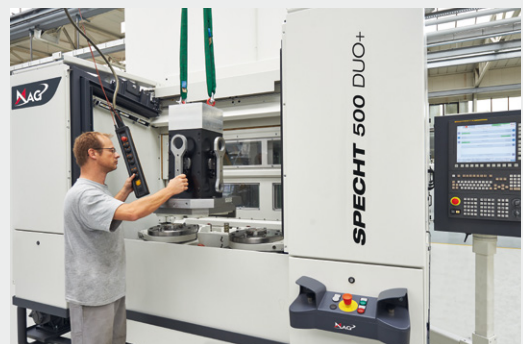
Easily accessible setup station on a SPECHT® 500 DUO+
