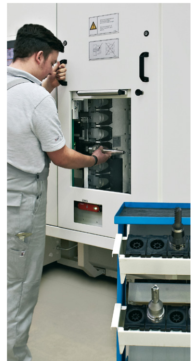
Tool magazine can be fitted during machining at ground level
