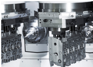
Overhead machining on a cylinder head on the SPECHT® DUO
