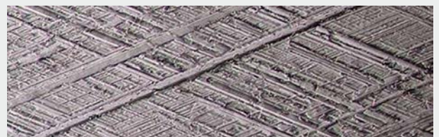
Magnification of a diamond-honed bore surface
