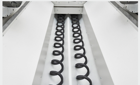
Chip tray with steep edges for good chip discharge also for MQL machining
