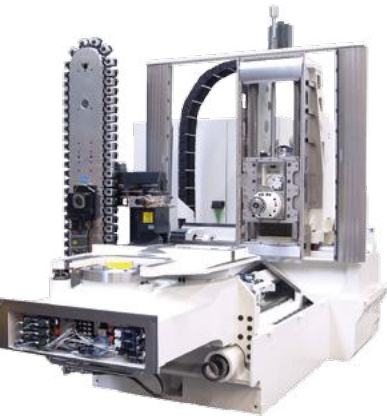
Basic structure of NBH 500 with geared spindle [option] and chain magazine with 60 tool locations [option]
