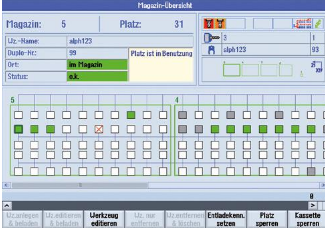
Clearly structured, graphical tool administration of the tool rack-type cassette magazine
