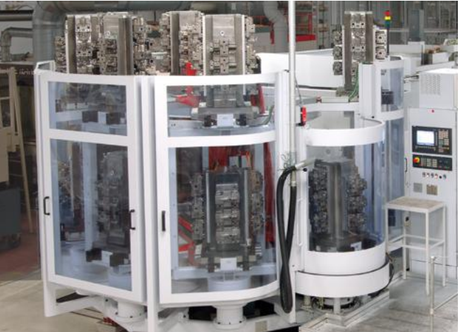
Very compact multi-pallet storage system (MPS) to deposit the pallets at 2 levels with space-saving installation surface for NBH 630.
