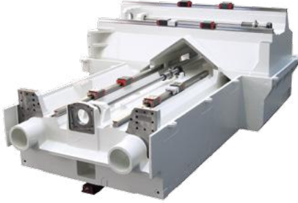
Compact, one-piece and rigid machine bed
