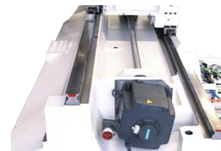
Two levels of X-axis guideways for maximum absorption of cutting forces
