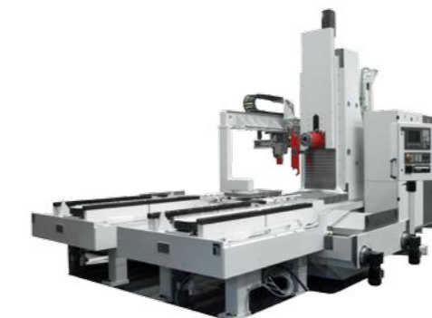
Basic structure of NBH 1200 with gantry-type column in Z-axis
