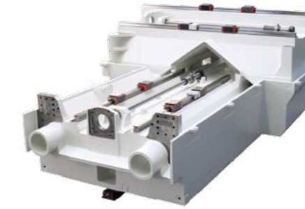
Compact, one-piece and rigid machine bed
