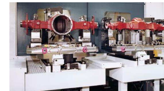
Failsafe loading/unloading of heavy workpieces utilizing a proven parallel linear pallet changer
