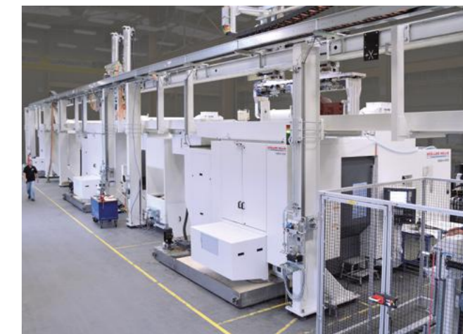
Part view of fully automatic manufacturing line for machining of gearboxes. Further details see text on the right.
