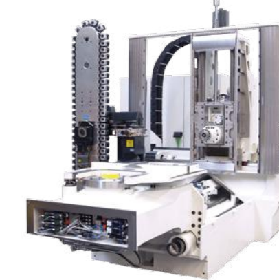
Basic structure of NBH 500 with geared spindle [option] and chain magazine with 60 tool locations [option]
