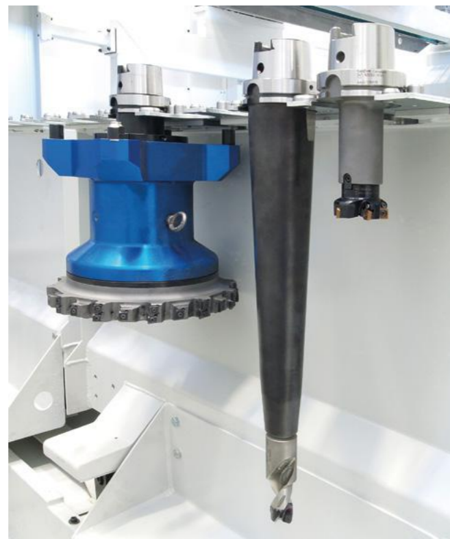
Interactive space requirement determination by the tool administration function. Ideal utilization of the tool magazine capacity by automatic collision observation of neighbouring locations on a millimeter basis
