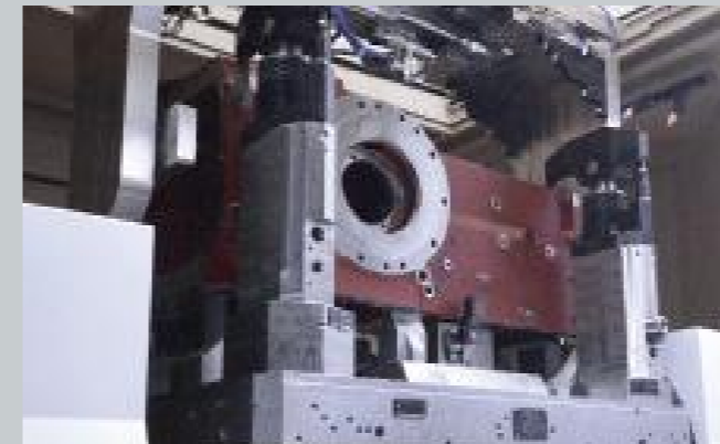
Direct loading of fixture on tilting/rotary table by means of 6-axis robot
