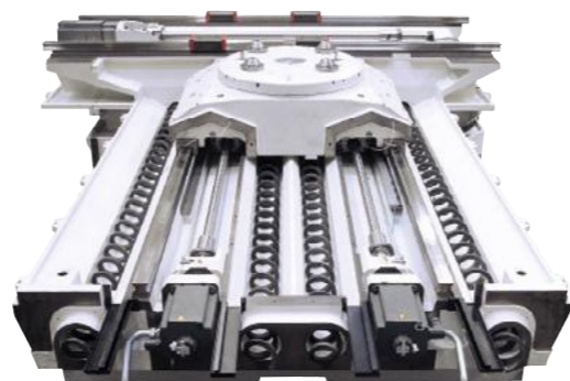
Machine bed with gantry drive in Z-axis and 4 integrated chip grooves for optimal chip removal
