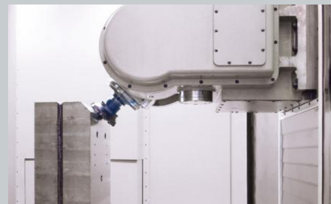
Milling machining with tilt head
