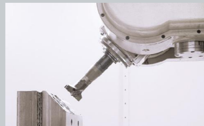
Drilling machining with tilt head
