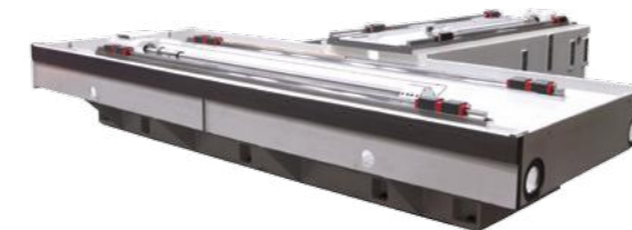
The X- and Z-bed are properly positioned and held together with a large-surface bolt connection
