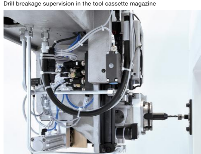
HÜLLER HILLE TOOL MANAGEMENT • Tool life quantities monitoring with automatic exchange for twin tools • In-process tool breakage monitoring in the tool magazine area
