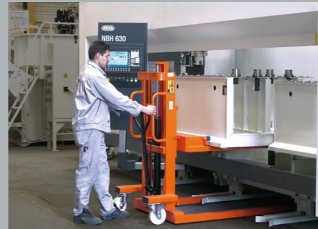
Enhanced machine utilization with the original rack-type cassette magazine for incycle changing sets of 50 tools by means of a cassette carriage in just a few minutes.
