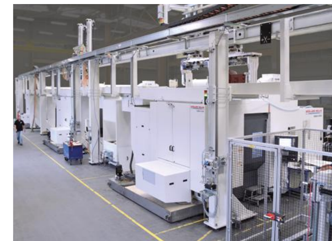
Part view of fully automatic manufacturing line for machining of gearboxes. Further details see text on the right.
