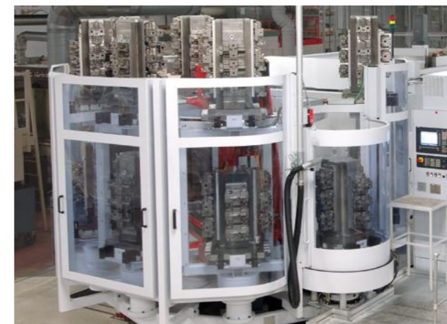
Very compact multi-pallet storage system (MPS) to deposit the pallets at 2 levels with space-saving installation surface for NBH 630.
