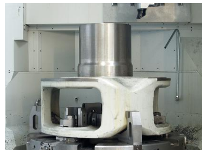
Machining of a planetary carrier
