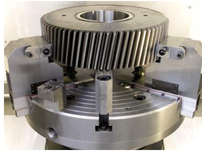
Gear wheel clamped on a VDM 550
