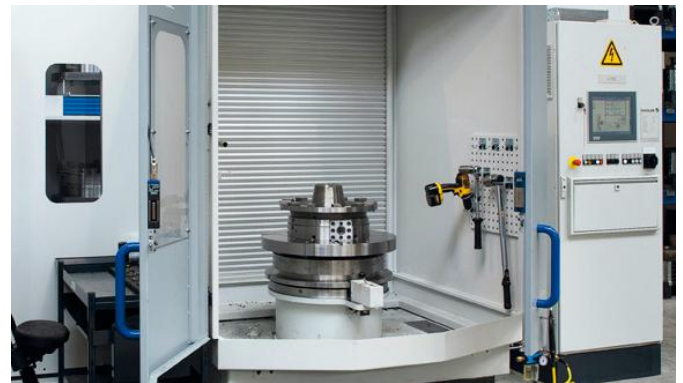
Pallet system with zero-point clamping
