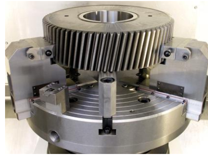
Gear wheel clamped on a VDM 550
