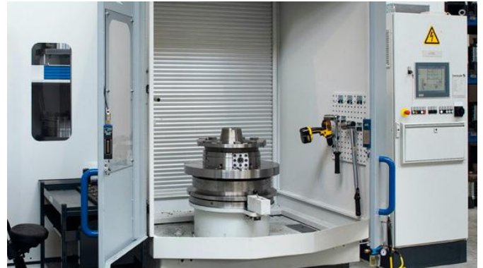
Pallet system with zero-point clamping
