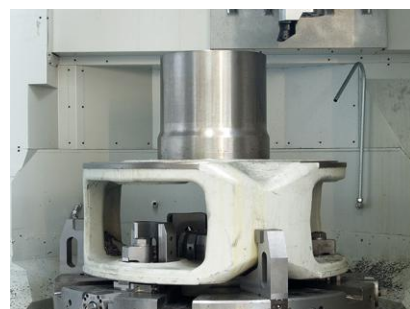
Machining of a planetary carrier
