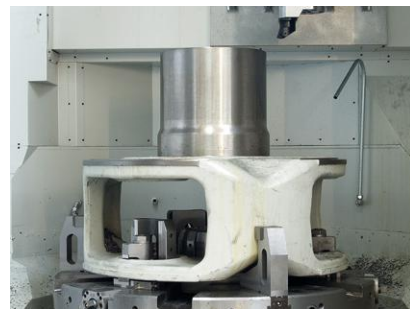
Machining of a planetary carrier
